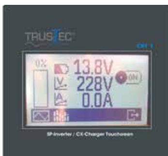
CRT1 touch screen for SP series inverters / CX chargers On / Off, display of all current flow values, battery capacity of BMS Dimensions 120 x 100 x 30 mm For technical data, see page 22
